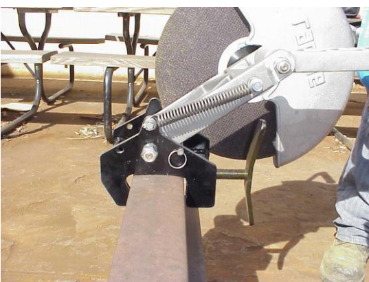
Rail Side Cutting with Operator's Position Adjacent to Clamp Tensioning Screw Stop Pin is inserted on operator's side.
