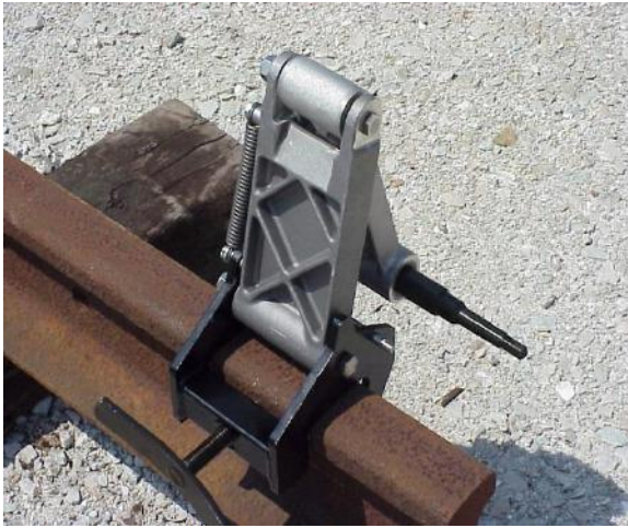
Rail Clamp Installed
