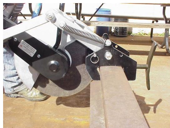
Rail Side Cutting with Operator's Position Opposite of Clamp Tensioning Screw Stop Pin is inserted on operator's side.
